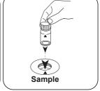
Fill 24 mm vial with 10 mL Close vial(s). sample.
