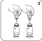
Add **3 drops Chloride-51 solution** to each vial.
