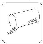
Rinse a beaker with the sample and empty it, leaving a few drops remaining in the beaker.
