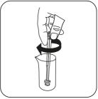
Crush tablet(s) by rotating slightly.
