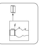
Remove **vial** from the sample chamber.
