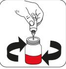
Add Alkalinity Reagent Reagent ALK4 drop by drop to the sample until colouration turns from colourless to red.
