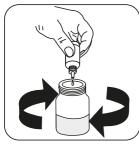
Add Alkalinity Reagent ALK3 or Alkalinity Reagent ALK4 drop by drop to the sample until discolouration turns from pink to colourless.
