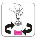
Add Carbon Dioxide LR Titrant CDX2 drop by drop to the sample until colouration turns from colourless to pink.
