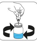
Add Hardness LR Titrant TH3 or Hardness HR Titrant TH4 drop by drop to the sample until colouration turns from wine red to blue.
