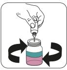
Add Polyacrylate HR Titrant A5 or Polyacrylate HR Titrant A6 drop by drop to the sample until colouration turns from blue to grey/ pink in the bottom layer.
