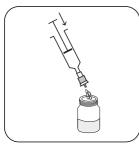
Filter sample with a filter (pore size 0.45 µm).
