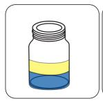
Allow phases to separate. A blue color should develop in the lower layer if any product is present.
