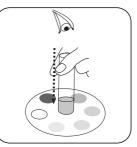
Look down through the tube, compare the colour produced in the tube to the colour standards printed on the comparison chart. Match to the nearest standard and read of the corresponding concentration value as Isothiazolinone in mg/l (ppm).
