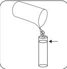
Fill up test tube with sample to the 10 mL mark.
