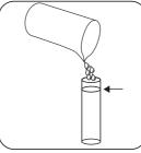
Fill up test tube with sample to the 10 mL mark.
