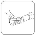
Close the daylight plate and press it lightly.
