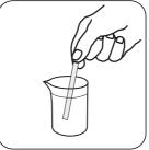
Remove one test strip. Hold Dip the test strip into the solution to be tested without agitation.
