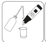
Rinse the electrode with distilled or deionised water and carefully wipe with a paper towel.
