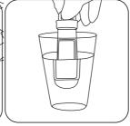
Sampling Fluids: The sample should be taken by immersing both sides of the paddle into the fluid to be tested.
