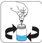
Add **Nitrite Titrant N2** drop by drop to the sample until colouration turns from **orange** to **blue**.
