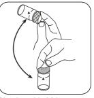
Dissolve tablet(s) by inverting.
