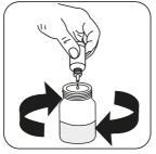
Add Alkalinity LR Titrant TA3 or Alkalinity HR Titrant PA2/TA2 drop by drop to the sample until discolouration turns from pink to colourless.
