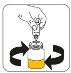
Add Alkalinity LR Titrant TA3 or Alkalinity HR Titrant PA2/TA2 drop by drop to the sample until colouration turns from blue to orange/yellow.
