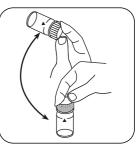
Dissolve tablet(s) by inverting.
