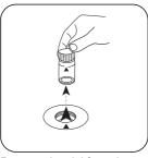
Remove the vial from the sample chamber.
