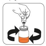
Add Chloride LR Titrant CC2 or Chloride HR Titrant BC2 drop by drop to the sample until colouration turns from yellow to orange/brown.
