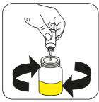
Add sufficient drops of **Phosphonate Neutraliser** P1/2 to give a yellow colour.
