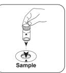
Fill 24 mm vial with 10 mL Close vial(s). prepared sample.
