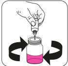
Add Hydrogen Peroxide HR Titrant HP2 or Hydrogen Peroxide LR Titrant HP3 drop by drop to the sample until colouration turns from colourless to pink.
