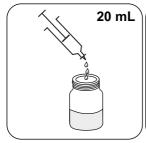
Fill the jar with 20 mL of the cooled sample.
