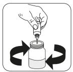
Add drops of Phosphonate Swirl to mix. pH Adjuster P3 until the sample is colourless.
