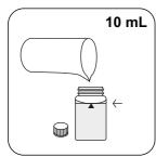
Fill 24 mm vial with 10 mL Close vial(s). deionised water.
