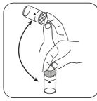
Dissolve tablet(s) by inverting.
