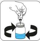
Add Sulphite Titrant S2 number of drops that will be drop by drop to the sample until colouration turns from colourless to blue.
