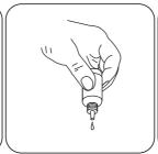
Add Hardness Calcium Buffer CH2 drop by drop to the same sample until colouration turns from light pink to red. (Note: make sure to swirl the vial after adding each drop!)
