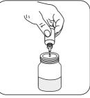
Add 4 drops of Hardness Calcium Buffer CH2 per 10 mL of sample.
