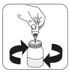
Add Alkalinity LR Titrant TA3 or Alkalinity HR Titrant PA2/TA2 drop by drop to the sample until discolouration turns from pink to colourless.
