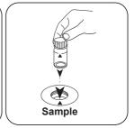
Fill 24 mm vial with **10 mL** Close vial(s). **sample**.
