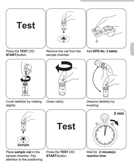
Once the reaction period is finished, the measurement takes place automatically.
