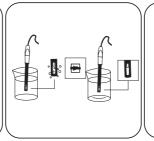
Immerse the measuring cell in the sample. During measurement, ensure that there are no air bubbles on the electrode surface and that the electrode, as well as the temperature sensor, are sufficiently surrounded by the sample. The measurement value can now be read off from the display. In the parameter configuration you can change the conductivity to TDS or salinity if required.
