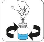
Add **Nitrite Titrant N2** drop by drop to the sample until colouration turns from **orange** to **blue**.
