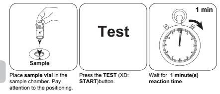
Once the reaction period is finished, the measurement takes place automatically.
