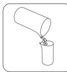
Fill a suitable digestion vessel with 50 mL homogenised sample.
