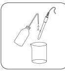
Rinse the electrode with distilled or deionised water and carefully wipe with a paper towel.
