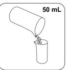
Add Hardness Calcium Buffer CH2 drop by drop to the same sample until colouration turns from light pink to red. (Note: make sure to swirl the vial after adding each drop!)
