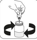
Add drops of **Phosphonate** Swirl to mix. **pH Adjuster P3** until the sample is colourless .
