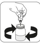
Add Alkalinity LR Titrant TA3 or Alkalinity HR Titrant PA2/TA2 drop by drop to the sample until discolouration turns from pink to colourless.
