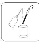
Rinse the electrode with distilled or deionised water and then with the sample.
