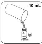
Fill 24 mm vial with **10 mL** prepared sample .
