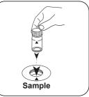
Fill 24 mm vial with **10 mL** Close vial(s). deionised water .
