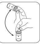
Dissolve tablet(s) by inverting.
