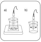
Immerse the pH electrode including temperature sensor in the calibration solution. Ensure sufficient flow, e.g. by a) use a magnetic stirrer with a stirring fish (recommended) b) Sway the pH electrode in the solution.
