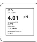
The pH value can be read in operating mode. Stop stirring while doing this.
