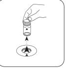
Remove the vial from the sample chamber.
