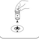
Remove the vial from the sample chamber.
