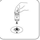
Remove the vial from the sample chamber.
