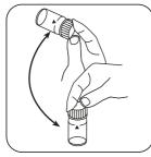
Dissolve tablet(s) by inverting.
