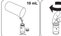
Fill 24 mm vial with **10 mL** Close vial(s). **prepared sample** .
