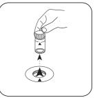
Remove the vial from the sample chamber.
