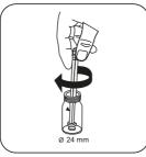
Crush tablet(s) by rotating slightly.
