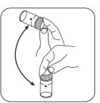
Crush tablet(s) by rotating slightly.
