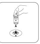
Remove the vial from the sample chamber.
