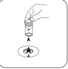
Remove the vial from the sample chamber.
