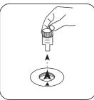
Remove **vial** from the sample chamber.
