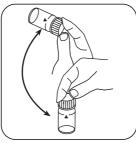
Dissolve tablet(s) by inverting.
