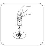
Remove the vial from the sample chamber.
