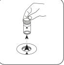
Remove the vial from the sample chamber.
