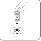
Remove the vial from the sample chamber.
