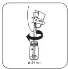
Crush tablet(s) by rotating slightly.
