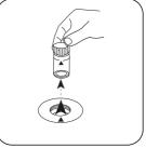
Remove the vial from the sample chamber.
