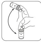
Dissolve tablet(s) by inverting.
