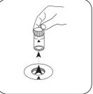
Remove the vial from the sample chamber.
