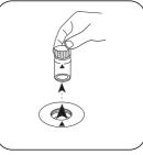
Remove the vial from the sample chamber.
