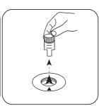
Remove vial from the sample chamber.
