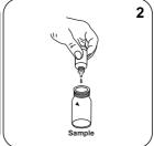
Add 2 drops DPD 1 Reagent Solution to the sample vial.
