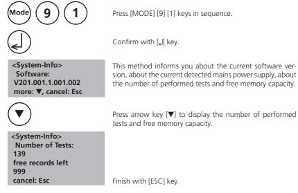
This method informs you about the current software version, about the current detected mains power supply, about the number of performed tests and free memory capacity.
