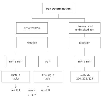
Digestion procedure for the determination of total dissolved and undissolved iron.
