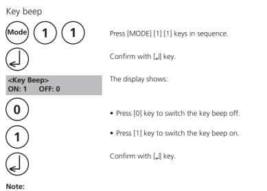
In the case of methods with reaction periods, an acoustic signal still sounds during the last 10 seconds of the countdown even if the key beep is switched off.
