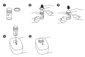
Correct position of the vial (Ø 16 mm):
