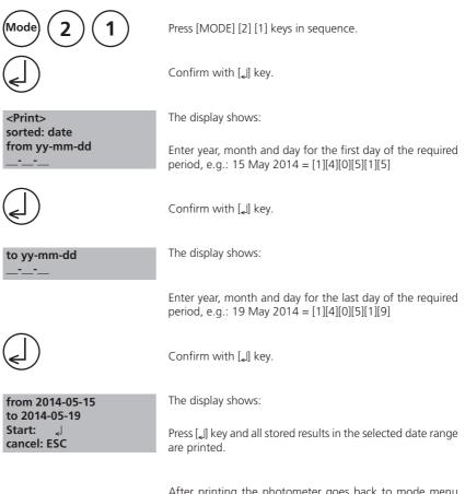
After printing the photometer goes back to mode menu automatically.
