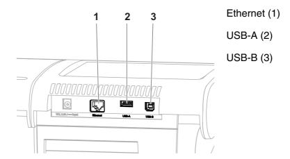
Figure 3-1 Communication interfaces on the rear panel
