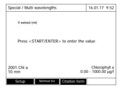
For methods with procedure variables: Enter the values of all procedure variables one after the other.
