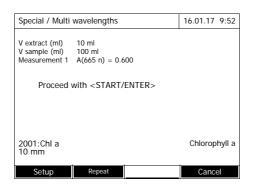
In case of several measurements, an intermediate result is displayed.
