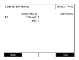
5 Insert the cell with the corresponding standard or reagent blank value (for E0).
