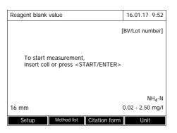
If necessary, make additional single measurements for the median value formation with [Next meas.] discard the last single measure-
