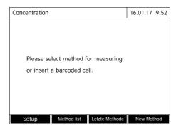
Inserting a cell with barcode starts a measurement.
