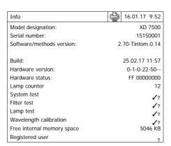
The meter information and result of the self-test are displayed and can be printed.
