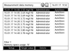
The Measurement data memory list is displayed. All measurement datasets corresponding to the filter criteria are hidden.
