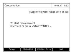
The photometer is ready to measure when all the required data have been confirmed or remeasured.
