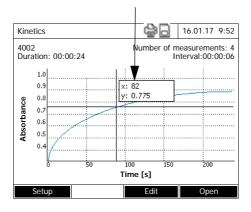
The cursor consists of a horizontal and a vertical line, which cross at a point of the curve. A box displays the x and y values of the curve point.
