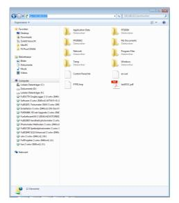
In Windows-Explorer on the PC, enter ftp://IP-address. The folders stored on the photometer are displayed.
