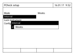
1 Enter a numeric value (2 to 52 weeks) (<0...9>) and confirm The *Interval* defined for the PCheck check is active.
