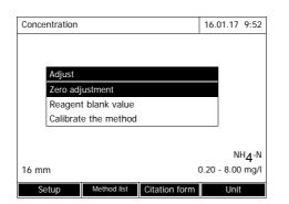
1 In the respective mode, press the <ZERO-BLANK> key.
