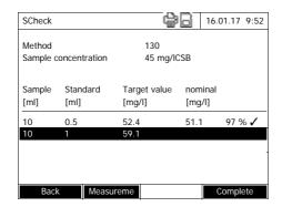
After the measurement, the recovery rate is displayed in the right table column.
