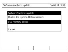
5 Using <▲><▼>, select USB memory device as the source and press <START-ENTER>.
