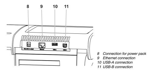
Figure 2-2 Rear panel with socket field
