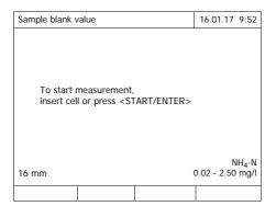
3 Insert the cell with a suitable blank sample.
