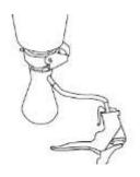
Attach filtration device to vacuum pump using tube
