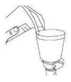
Pour sample into the filtration device
