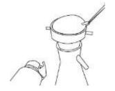
Place filter into filtration device
