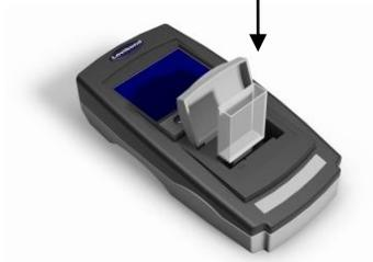
7 - Close the sample lid and press the test key on the keypad or the display.
