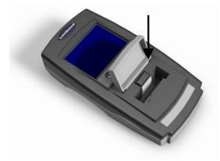
3 - Close the sample lid and press the zero key on the keypad or the display.
