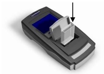
3 - Close the sample lid and press the test key on the keypad or the display.
