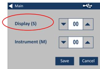
5b – Press the up and down arrows to set the time interval before the instrument shuts down after being inactive.
