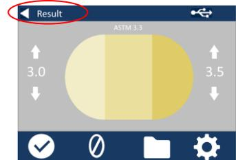
8 - Press the up and down arrows to view the stages / steps as they would be on the visual disc.
