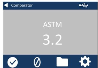
5- Press the back arrow on the display to change between numeric and comparator mode
