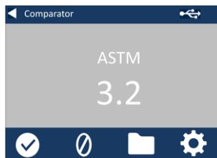
10 - Compare the result from the instrument to the value on the label of the validation liquid, to check it is within the specified tolerances.
