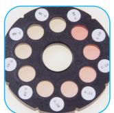
The table on the following pages provides details of the commonly used Lovibond® test discs that are available for water analysis.
