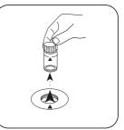
Remove the vial from the sample chamber.
