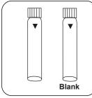
Prepare two digestion vials TN Hydroxide LR Mark one as a blank.
