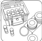
After sampling, the dipslides should be placed immediately into incubation at 30 - 35 °C for 24 - 48 hours. For fungi and moulds incubate for up to 5 days.
