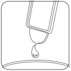
Excess sample should be gently shaken from the paddle before it is replaced in the container.
