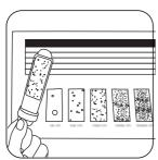
After incubation compare result of the dipslide to the dipslide comparison chart to quantify the result. For documentation and evaluation, you can also use our "Diplside Comparator 2" App.
