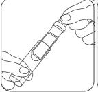
Place the dipslide back into the container while holding on the outer cover.
