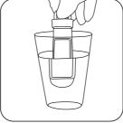
Sampling Fluids: The sample should be taken by immersing both sides of the paddle into the fluid to be tested.
