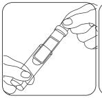
Remove the dip slide from the container by pulling the white tap while holding on to the outer cover.
