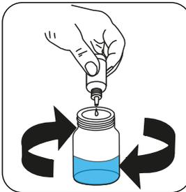
Add **Hardness LR Titrant TH3** or **Hardness HR Titrant TH4** drop by drop to the sample until colouration turns from **wine red** to **blue**.
