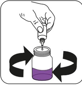
Add **Phosphonate Titrant P5** drop by drop to the sample until colouration turns through **grey** to **purple**.
