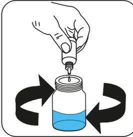
Add **Sulphite Titrant S2** drop by drop to the sample until colouration turns from **colourless to blue**.
