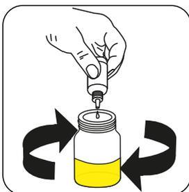
Add **sufficient** drops of **Phosphonate Neutraliser P1/2** to give a **yellow** colour.
