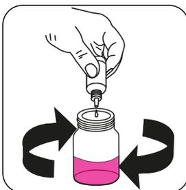
Add **Hydrogen Peroxide HR Titrant HP2 or Hydrogen Peroxide LR Titrant HP3** drop by drop to the sample until colouration turns from **colourless** to **pink**.
