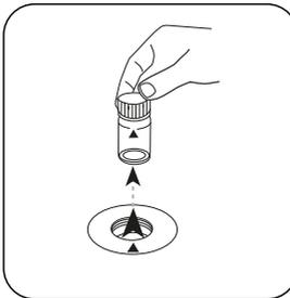
Remove the vial from the sample chamber.
