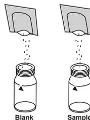
Add a **Monochlor FRGT powder pack** simultaneously in each vial.
