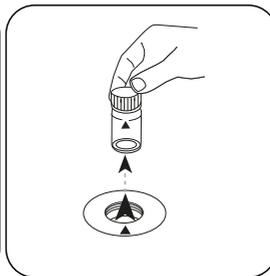
Remove the vial from the sample chamber.
