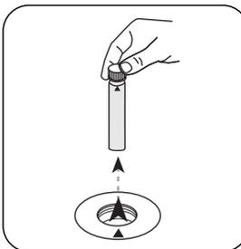
Remove **vial** from the sample chamber.
