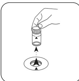
Remove the vial from the sample chamber.
