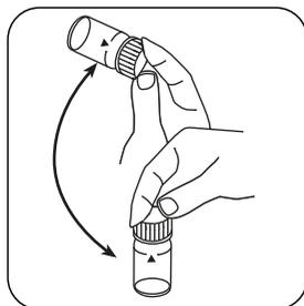
Invert several times to mix the contents (for at least 60 s until the tablet is completely dissolved).
