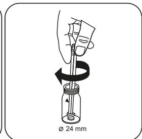
Crush tablet(s) by rotating slightly.
