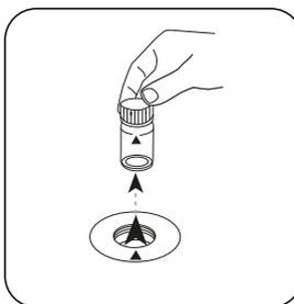
Remove the vial from the sample chamber.
