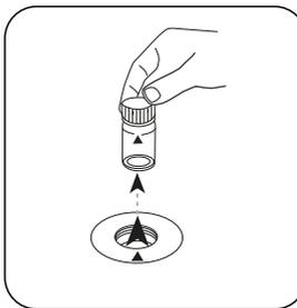
Remove the vial from the sample chamber.
