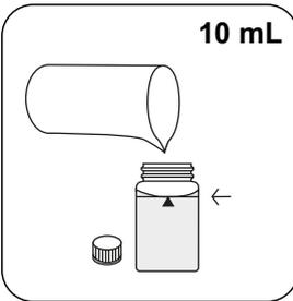
Fill 24 mm vial with **10 mL sample**. Close vial(s).
