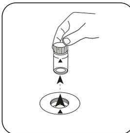
Remove the vial from the sample chamber.
