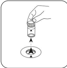
Remove the vial from the sample chamber.
