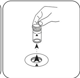
Remove the vial from the sample chamber.
