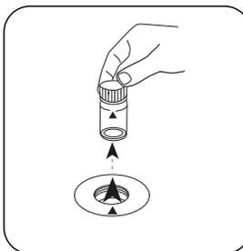
Remove the vial from the sample chamber.
