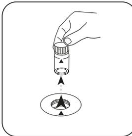
Remove the vial from the sample chamber.
