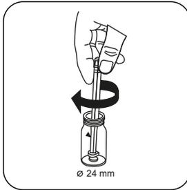
Crush tablet(s) by rotating
