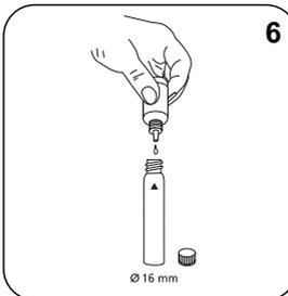
Add **6 drops H<sub>2</sub>O<sub>2</sub>-Reagent Solution**.
