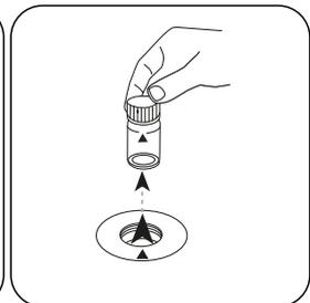
Remove the vial from the sample chamber.
