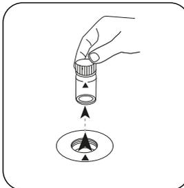
Remove the vial from the sample chamber.
