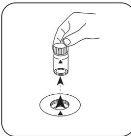
Remove the vial from the sample chamber.
