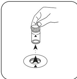
Remove the vial from the sample chamber.
