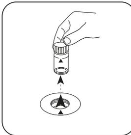
Remove the vial from the sample chamber.
