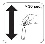
Mix the contents by shaking Seal the vials in the previgorously. (> 30 sec.).
