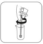
Crush tablet(s) by rotating slightly.
