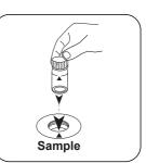
Add exactly 10 ml sample Close vial(s). to the 450 mm vial.
