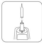
Place Zero ampoule in the sample chamber.
