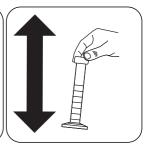
Stopper the mixing cylinder. Shake to dissolve the powder.
