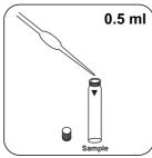
Fill sample vial with 0.5 ml Close vial(s). prepared, digested sample.
