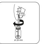
Add AMMONIA No.1 tablet Crush tablet(s) by rotating slightly.
