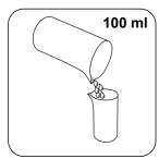
Fill a suitable sample vessel with 100 ml sample sulfuric acid (≥ 95 %).
