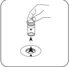
Remove the vial from the sample chamber.
