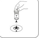
Remove the vial from the sample chamber.
