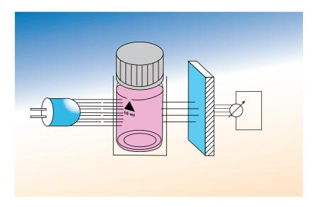
Transmission is the ratio of the intensity of light before (I0) and after (I) radiating freely through the sample. To represent this absorption of light over a large area, a negative common logarithm of the transmission is usually chosen, which is also known as extinction or absorbency.
