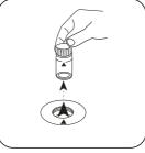
Remove the vial from the sample chamber.
