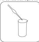
In the sample vessel, put 2 ml sample and 8 ml deionised water .
