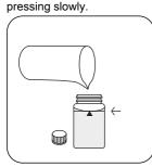
Fill up vial with sample to the 10 ml mark.
