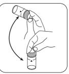
Crush tablet(s) by rotating slightly.
