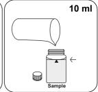
Fill sample vial with 10 ml prepared, digested sample.
