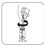
Crush tablet(s) by rotating slightly.
