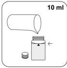
Place 10 ml Nitrite VHR L Close vial(s). solution in the test vial.
