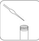
Fill a Nitratest tube with **20 ml sample**.
