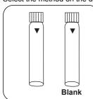
Prepare two reaction vials. Put 2 ml deionised water Mark one as a blank.
