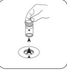
Remove the vial from the sample chamber.
