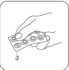
Add CHLORIDE T2 tablet . Crush tablet(s) by rotating
