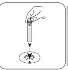
Place sample vial in the sample chamber. • Pay attention to the positioning. The result in mg/I  $H_2O_2$  appears on the display.
