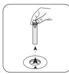
Remove **vial** from the sample chamber.
