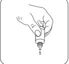
Hold cuvettes vertically and add equal drops by pressing slowly.
