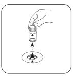
Remove the vial from the sample chamber.
