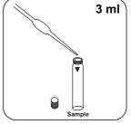
Prepare two reaction vials. Place 3 ml of prepared Mark one as a blank.
