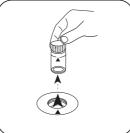
Remove the vial from the sample chamber.
