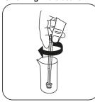
Crush tablet(s) by rotating slightly.
