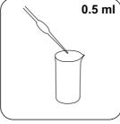
Place **0.5 ml Reagenz Pb-1** in a suitable sample vessel.
