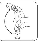
Dissolve tablet(s) by inverting.
