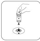
Remove the vial from the sample chamber.
