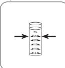
Fill the sample glass to the 25 ml mark with the sample.
