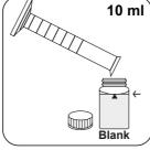
Fill blank with 10 ml prepared sample.
