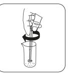
Dissolve the tablets using a clean stirring rod.
