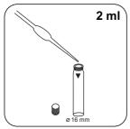
Add 2 ml 1,00 N Sodium Hydroxide solution to the digested sample.
