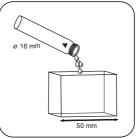
Fill 50 mm vial with prepared sample.
