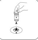
Remove the vial from the sample chamber.
