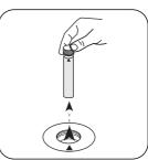
Place the supplied Zero vial Press the ZERO button. (red sticker) in the sample chamber. • Pay attention to the positioning.
