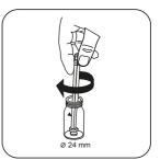
Crush tablet(s) by rotating slightly.
