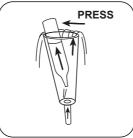
Place a Vacu-vial® ampoule in the sampling vessel. Break off the ampoule tip by applying light pressure against the vessel wall. Wait for the ampoule to fill completely.
