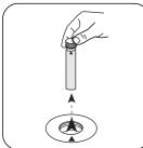
Remove **vial** from the sample chamber.
