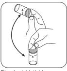
Dissolve tablet(s) by inverting.
