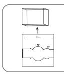
Remove **vial** from the sample chamber.
