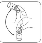
Dissolve tablet(s) by inverting.
