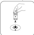
Remove the vial from the sample chamber.
