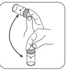
Dissolve tablet(s) by inverting.
