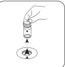
Remove the vial from the sample chamber.
