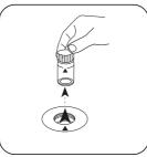
Remove the vial from the sample chamber.
