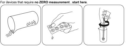
Rinse a beaker with the sample and empty it, leaving a few drops remaining in the beaker.
