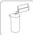
Return the sample solution Add DPD No.3 HR tablet. completely to the sample vessel.
