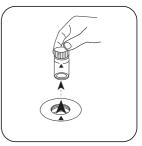
Remove the vial from the sample chamber.
