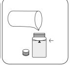
Fill up vial with sample to the 10 ml mark.
