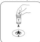
Remove the vial from the sample chamber.
