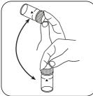
Dissolve tablet(s) by inverting.
