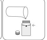
Fill up vial with **sample** to the **10 ml mark**.
