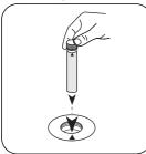
Place the supplied Zero vial Press the **ZERO** button. (red sticker) in the sample chamber. • Pay attention to the positioning.
