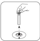
Remove **vial** from the sample chamber.
