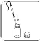
Keep the UV lamp in the sample. Note: wear UV safety goggles!
