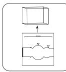
Remove vial from the sample chamber.
