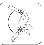
Crush tablet(s) by rotating slightly.
