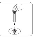
Remove vial from the sample chamber.
