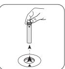
Remove **vial** from the sample chamber.
