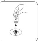
Remove the vial from the sample chamber.
