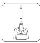
Place the ampoule in the sample chamber.
