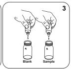
Add **3 drops Chloride-52 solution** to each vial.
