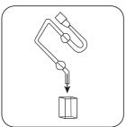
Fill 20 mm vial with the coloured absorption solu-
