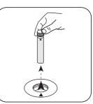
Remove **vial** from the sample chamber.
