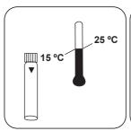
Allow the sample to cool to Open the vial. room temperature.
