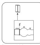
Remove **vial** from the sample chamber.
