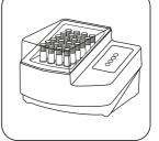
Warm vial for 120 minutes at 120 °C in a pre-heated thermoreactor in inverted position.
