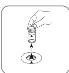
Remove the vial from the sample chamber.
