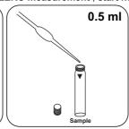
Fill sample vial with 0.5 ml Close vial(s). prepared, digested sample.
