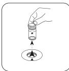
Remove the vial from the sample chamber.
