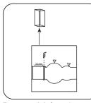
Remove **vial** from the sample chamber.
