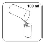
Fill a suitable sample vessel with 100 ml sample sulfuric acid (≥ 95 %).
