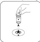
Remove the vial from the sample chamber.
