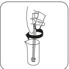
Crush tablet(s) by rotating slightly.
