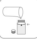
Fill up vial with deionised water to the 10 ml mark .
