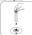
Remove **vial** from the sample chamber.
