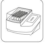
Seal the vials in the preheated thermoreactor for 30 minutes at 100 °C.
