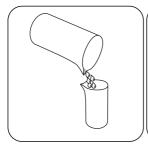
Fill a suitable digestion vessel with 50 ml homogenised sample.
