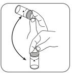
Dissolve tablet(s) by inverting.
