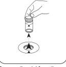
Remove the vial from the sample chamber.
