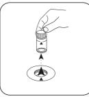
Remove the vial from the sample chamber.
