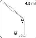
Put **4.5 ml deionised** water in the digestion vial.
