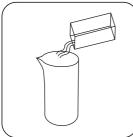
Return the sample solution Add DPD No. 3 tablet . completely to the sample vessel.
