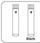
Prepare two digestion vials TN Hydroxide HR. Mark one as a blank.
