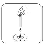
Remove **vial** from the sample chamber.
