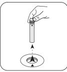
Remove vial from the sample chamber.
