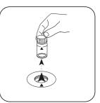
Remove the vial from the sample chamber.
