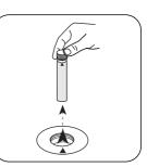
Remove **vial** from the sample chamber.
