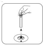
Remove **vial** from the sample chamber.
