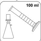
Filter approx. 100 ml sample with a pre-rinsed filter (pore size 0.45 μm).
