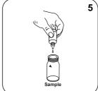
Add 5 drops Free Chlorine Reagent Solution to the sample vial.
