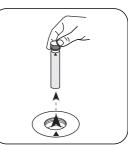
Remove vial from the sample chamber.
