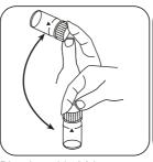
Dissolve tablet(s) by inverting.
