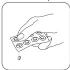
Add SULFIDE No. 1 tablet Crush tablet(s) by rotating
