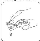
As an alternative to DPD No. 1 and No. 3 tablets, a DPD No. 4 tablet can be added.
