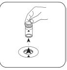
Remove the vial from the sample chamber.
