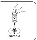
Put **2 ml sample** and **8 ml** Close vial(s). **of deionised water** in the sample vessel.
