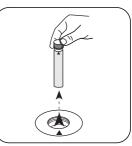
Remove **vial** from the sample chamber.
