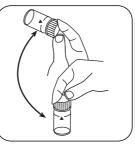
Dissolve tablet(s) by inverting.
