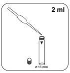
Add 2 ml 1,54 N Sodium Hydroxide Solution to the digested sample.
