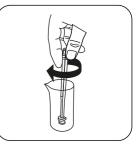
Crush tablet(s) by rotating slightly and dissolve.
