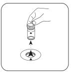
Remove the vial from the sample chamber.
