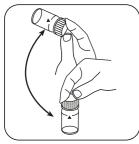
Dissolve tablet(s) by inverting.
