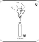
Add 6 drops H<sub>2</sub>O<sub>2</sub>-Reagent Solution.
