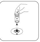
Remove the vial from the sample chamber.
