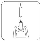
Place **Zero ampoule** in the sample chamber.
