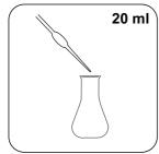
Put 20 ml homogenised sample in the erlenmeyer flask.
