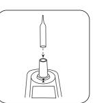
Remove zero ampoule from the sample chamber.
