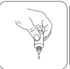
Add KS 144 (Calcium Hardness Buffer) drop by drop to the same sample until colouration turns from light pink to red. (Note: make sure to swirl the vial after adding each drop!)
