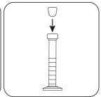
Stopper the mixing cylinder. Swirl around to dissolve the powder.
