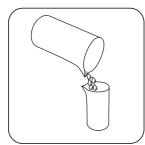
Fill a suitable digestion vessel with 50 ml homogenised sample.
