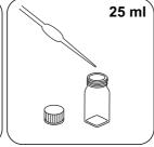
Fill one of the digestion vials with 25 ml of prepared sample.
