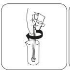
Crush tablet(s) by rotating slightly and dissolve.
