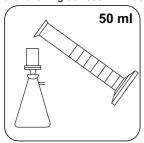
Filter approx. 50 ml sample Fill 50 mm vial with with a pre-rinsed filter (pore deionised water. size 0.45 µm).
