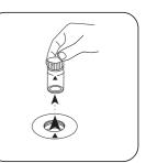
Remove the vial from the sample chamber.
