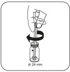
Crush tablet(s) by rotating slightly.
