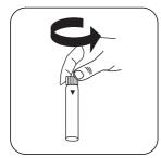
Open a digestion vial PO<sub>4</sub>-P Acid Reagent.
