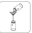
Any slight turbidity that occurs must be removed by filtration.
