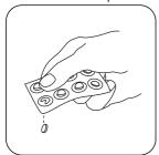
Add CALCIO H No.1 tablet Crush tablet(s) by rotating
