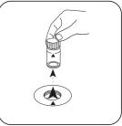
Remove the vial from the sample chamber.
