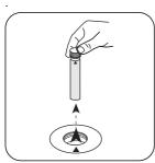
Remove **vial** from the sample chamber.
