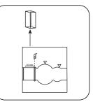
Remove vial from the sample chamber.
