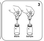
Add **3 drops Chloride-51 solution** to each vial.
