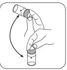
Dissolve tablet(s) by inverting.
