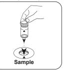
Swirl around to dissolve the Place sample vial in the sample chamber. • Pay attention to the positioning.
