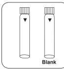
Prepare two digestion vials TN Hydroxide LR. Mark one as a blank.
