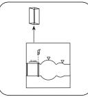
Remove **vial** from the sample chamber.
