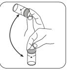
Dissolve tablet(s) by inverting.
