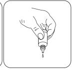
Add KS 144 (Calcium Hardness Buffer) drop by drop to the same sample until colouration turns from light pink to red. (Note: make sure to swirl the vial after adding each drop!)
