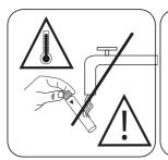
Allow vial to stand inverted for 1 hour and to cool. **Do not cool it with water!** After cooling down, rotate it and measure in the photometer **within 10 min**
