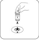
Remove the vial from the sample chamber.
