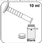
Fill blank with 10 ml prepared, not digested sample.
