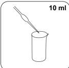
Fill a suitable sample vessel with 10 ml sample . .
