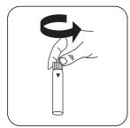
Open a digestion vial PO<sub>4</sub>-P Acid Reagent.
