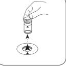
Remove the vial from the sample chamber.
