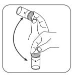
Dissolve tablet(s) by inverting.
