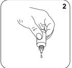
Add 2 drops KS135 (Phenolphthalein Substitute Indikator).
