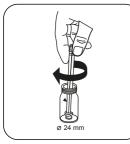
Crush tablet(s) by rotating slightly.
