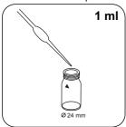
Place 1 ml (25 Tropfen) KS255 (Polyacrylate Reagenz 1) solution in the test vial.
