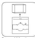
Remove **vial** from the sample chamber.
