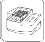
Seal the vials in the preheated thermoreactor for 60 minutes at 100 °C.
