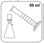
Filter approx. 50 ml sample Put 10 ml deionised with a pre-rinsed filter (pore water in the blank. size 0.45 µm).
