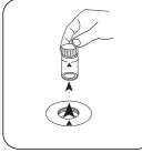
Remove the vial from the sample chamber.
