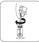
Crush tablet(s) by rotating slightly.
