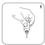
Add 1 drops KS135 (Phenolphthalein Substitute Indikator).
