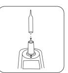
Remove zero ampoule from the sample chamber.
