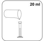
Put 20 ml sample in 25 ml Add Vario Molybdenum measuring cylinder
