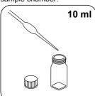
Fill a suitable sample vessel with 10 ml sample. date Reagent.
