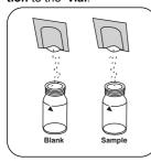
Add a Monochlor FRGT powder pack simultaneously in each vial.
