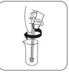
Fill a suitable sample vessel with **10 ml sample**.
