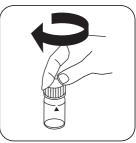
Filter approx. 14 ml sample Fill 24 mm vial with 10 ml with a pre-rinsed filter (pore prepared sample. size 0.45 µm).
