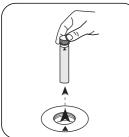
Remove **vial** from the sample chamber.
