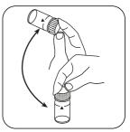
Dissolve tablet(s) by inverting.
