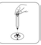
Place sample vial in the sample chamber. • Pay attention to the positioning. The result in mg/l Nitrogen appears on the display.
