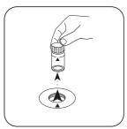
Remove the vial from the sample chamber.
