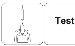
Place the ampoule in the sample chamber.
