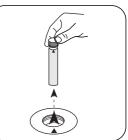
Place blank in the sample Press the ZERO button. chamber. • Pay attention to the positioning.
