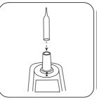
Place the ampoule in the sample chamber.
