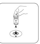
Remove the vial from the sample chamber.
