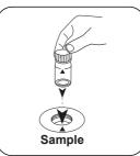
Place sample vial in the attention to the positioning. The result in mg/l free Chlorine appears on the display.
