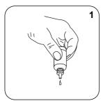
Add 1 drops KS135 (Phenolphthalein Substitute Indikator).
