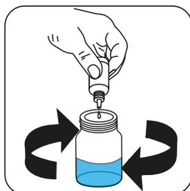
Add **Chlorine Free LR Titrant FCL2 or Chlorine Free HR Titrant FCL3** drop by drop to the sample until colouration turns from **colourless/pale yellow to blue**.
