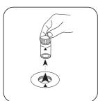
Remove the vial from the sample chamber.
