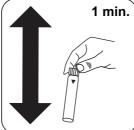
Mix the contents by shaking Press the ENTER button. vigorously. (1 min.).
