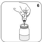
Add 6 drops Free Chlorine Buffer FCL1. Note: Add 10 drops when hardness of sample is greater than 400 mg/l (as CaCO<sub>3</sub>).
