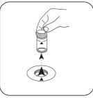
Remove the vial from the sample chamber.
